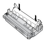
**9** Turn the two levers (①) on the toner cartridge firmly.
